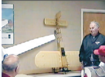
Richard Malinowski brought his 29" wingspan bee. It is powered with a Norvel .061 and has a wing loading of 5.5 ounces per square foot (on the picture his son Matt is showing the Bee)
