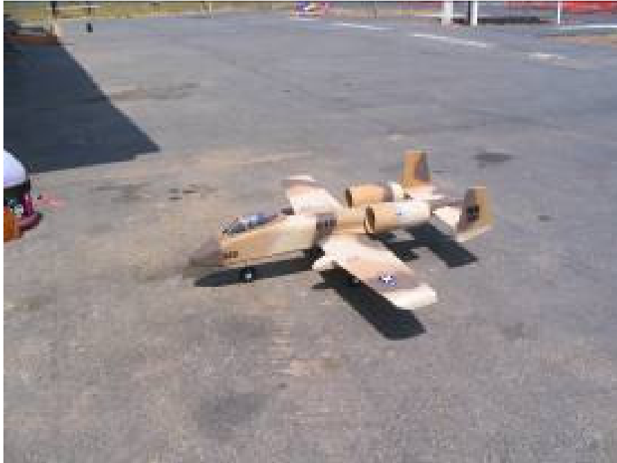
Richards's semi custom electric ducted fan. It flew much better once he put in stronger batteries and fixed the ESC so that he had full throttle.
